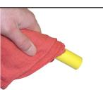
**3** Clean piping thoroughly to assure there is no dirt, grease or oil in assembly area.
