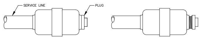
**3** Once venting is complete, remove plug by turning plug in a counterclockwise direction.
